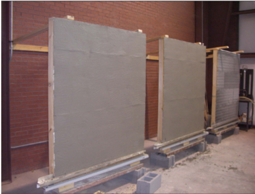
Water Penetration Panels (Photo 1)
