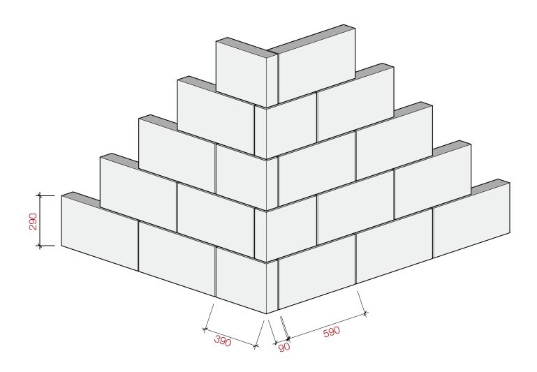
Developed for efficiency, our new 390 mm long Renaissance® corner unit makes it easier to maintain a half bond in a wall. Our field tests have shown as much as a 50% reduction in overall cutting; saving time and equipment.
