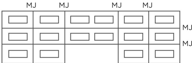
These joints are used to prevent cracking in the brick as they and the other materials along the perimeter of the building move at different rates and directions. The determination as to where to place movement joints is based on the material and building movements. It is then possible to evaluate where the movement joints need to be placed.
