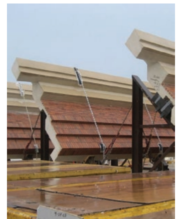
Thin brick panels ready for delivery to job site
